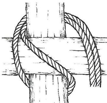
The Mark II Japanese Square Lashing is tied by looping the center of the rope of the upright spar and then forming the wrapping turns by taking the ends of the rope in opposite directions.
