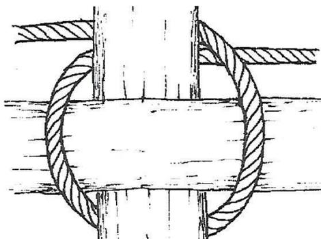
The Mark III is the same as the Mark II but a clove hitch is tied around the up right spar when starting the lashing.
