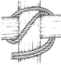
The Mark II Japanese Square Lashing is tied by looping the center of the rope of the upright spar and then forming the wrapping turns by taking the ends of the rope in opposite directions.
