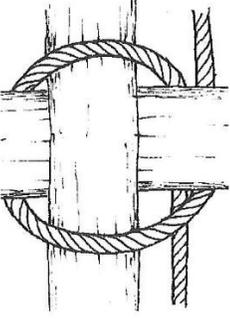
The Mark III is the same as the Mark II but a clove hitch is tied around the upright spar when starting the lashing.
