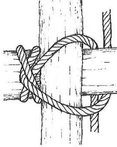
The Mark III is the most secure of the three Japanese square lashings because the clove hitch helps to prevent the lashing from shifting along the vertical spar.
